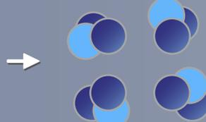
The oxygen, hit by the electric discharge, reacts transforming itself into ozone
